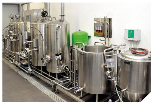
Experimental brewery, technological line for the production of beer
