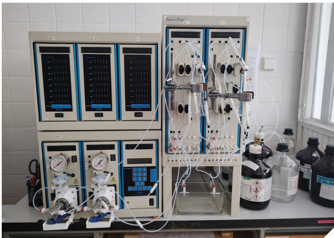
PowerPrep - purification of extracts
