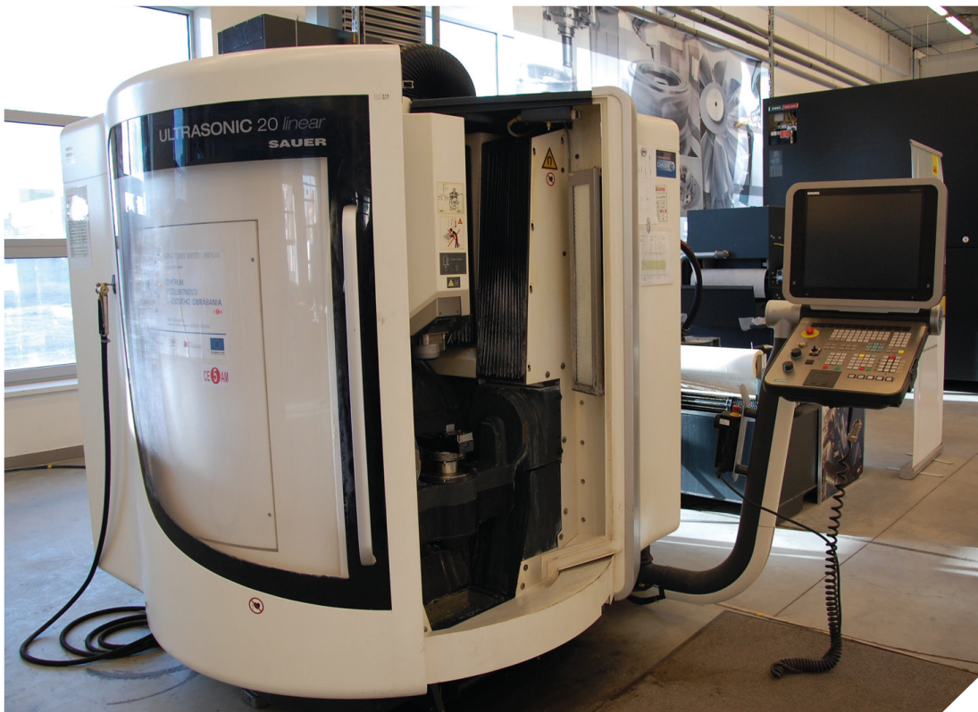
Center of excellence's 5-axis CNC machine HSC Ultrasonic 20 linear- 5-axis milling center with ultrasound support
